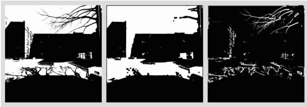
Figure 28: High-frequency filtering. Left : boolean image corresponding to image on figure 27 - Middle : high-frequency detection (dilatation-erosion) - Right : edge mask. Most of the noisy edges have been detected.
