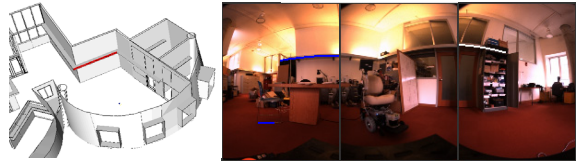
Figure 17. Putative correspondence determined by INIT-SEGMENT-EDGE. The algorithm determines the highest-scoring matches for the model segment (in red on the left) among the observed image edges. The three best candidates are displayed on the right. The correct match appears in blue on the left-hand side.
