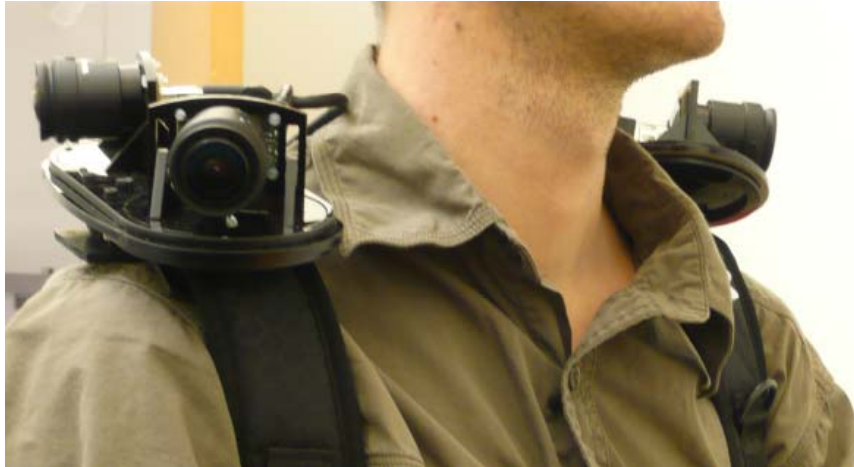
Four IEEE1394 PointGrey Firefly Cameras 4 x 360 x 240 SIFT detection & tracking at 4Hz FOV: 360° (h) x 90° (v)
