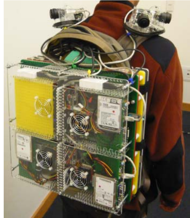
Embedded PC cluster Three 1.8Ghz Intel Core 2 Duo 3h untethered operation
